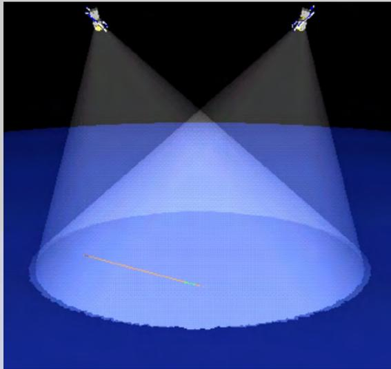
Use the **stereo** air fluorescence technique to image 325 → 425 nm photons in  $\sim 0.06^\circ$  pixels ( $\sim 1 \text{ km}^2$  projected on the ground) using 100 ns readout, from low Earth, **equatorial** ( $5 - 10^\circ$  inc.) orbit, induced by airshowers: **Original OWL Concept:  $E_{\text{th}} \approx 3 \times 10^{19} \text{ eV}$**
