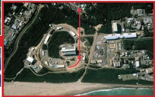
3. Off-axis ( $2.5^\circ$ ) beam travels 295km through earth to SK.
