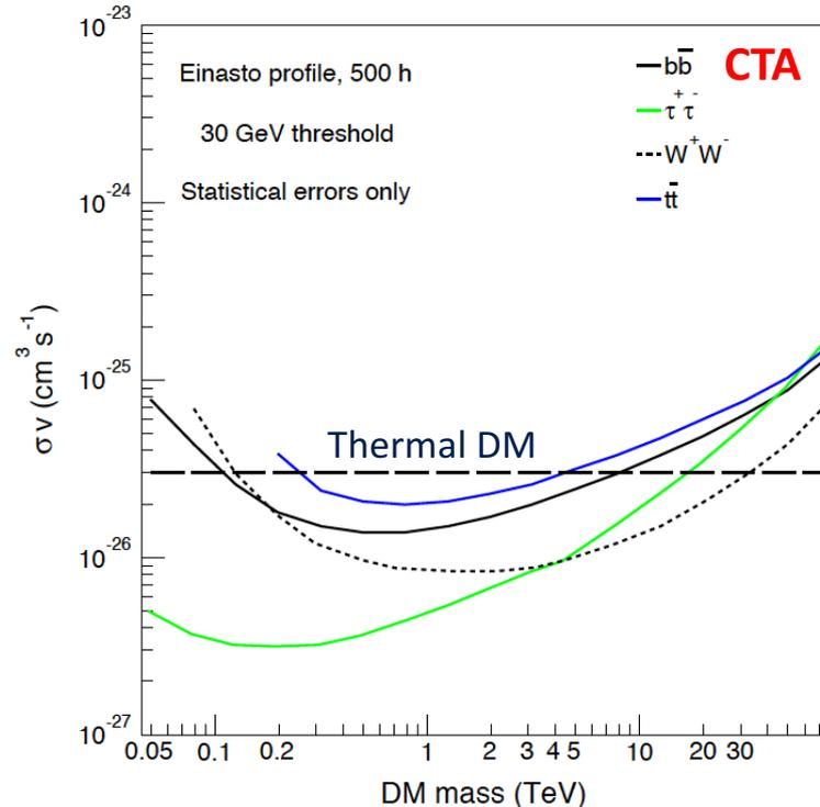
CTA will probe, *at the level of the thermal relic cross section*, WIMP masses and couplings not accessible to the LHC or direct detection
