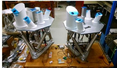
pSCT global alignment system: optical tables fabricated, undergoing calibration
