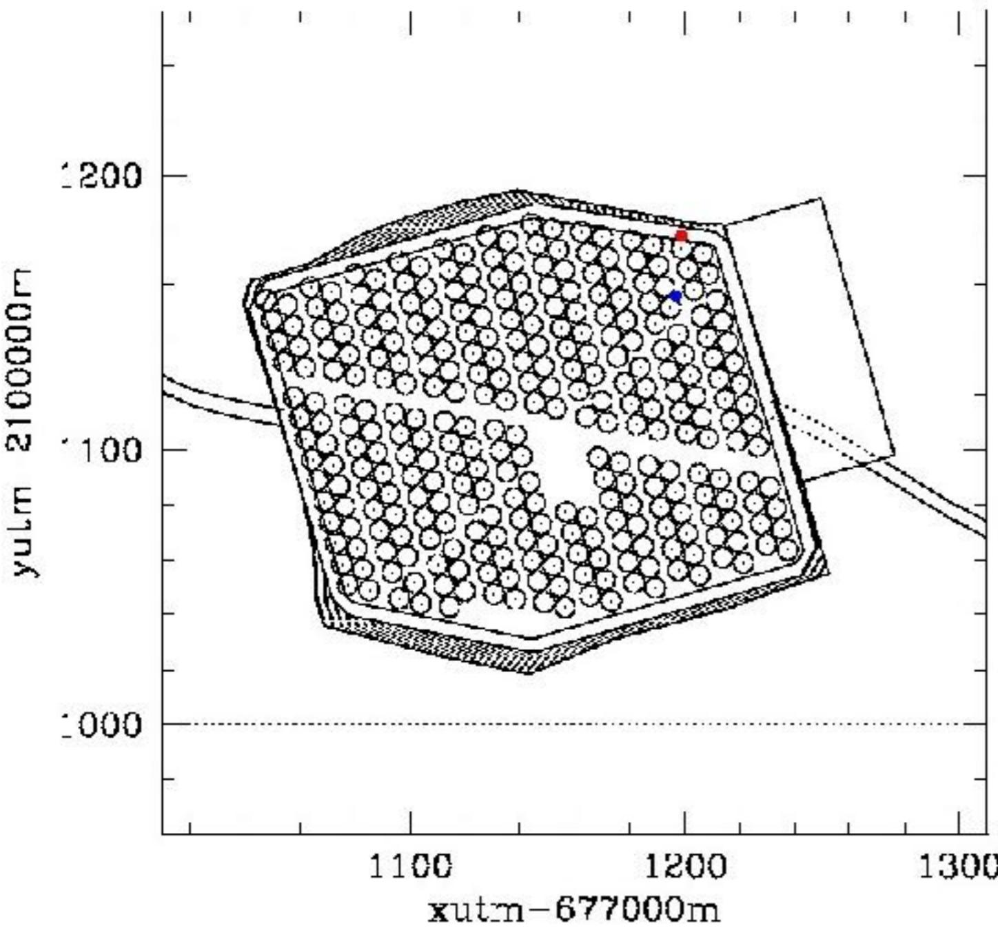
Array of 300 individual WCDs with 3+1 PMTs each = 1,200 PMTs.
