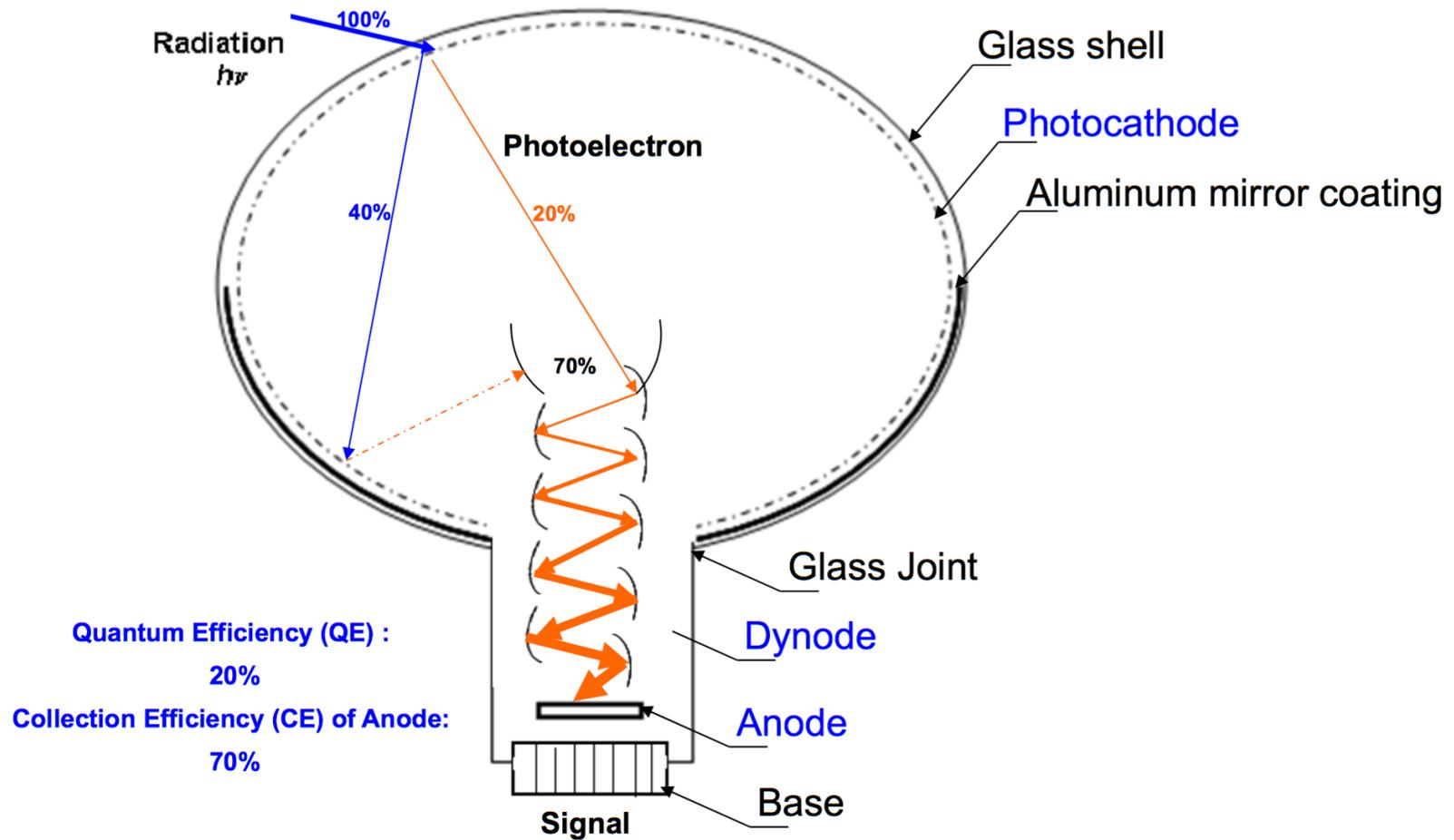
$$\text{Photon Detection Efficiency (PE)} = \text{QE}_{\text{Trans}} * \text{CE} = 20\% * 70\% = 14\%$$
