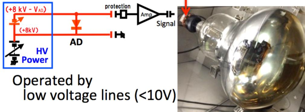
External HV Option → Confirmed with 100 m HV extension
