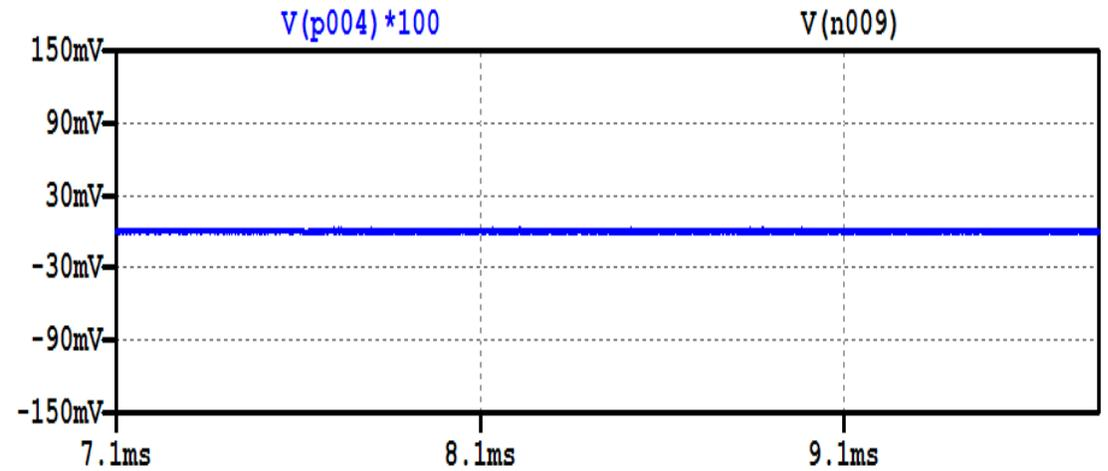
Switching supply (LT8611) residue at input of amp, scaled by amp gain
