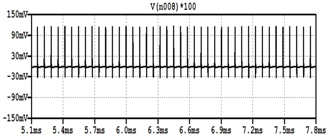
Switching supply (LMZ12001) residue at input of amp, scaled by amp gain
