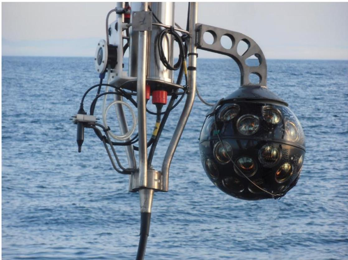
**PPM-DOM:** A prototype DOM on an Antares line (2500 m)
