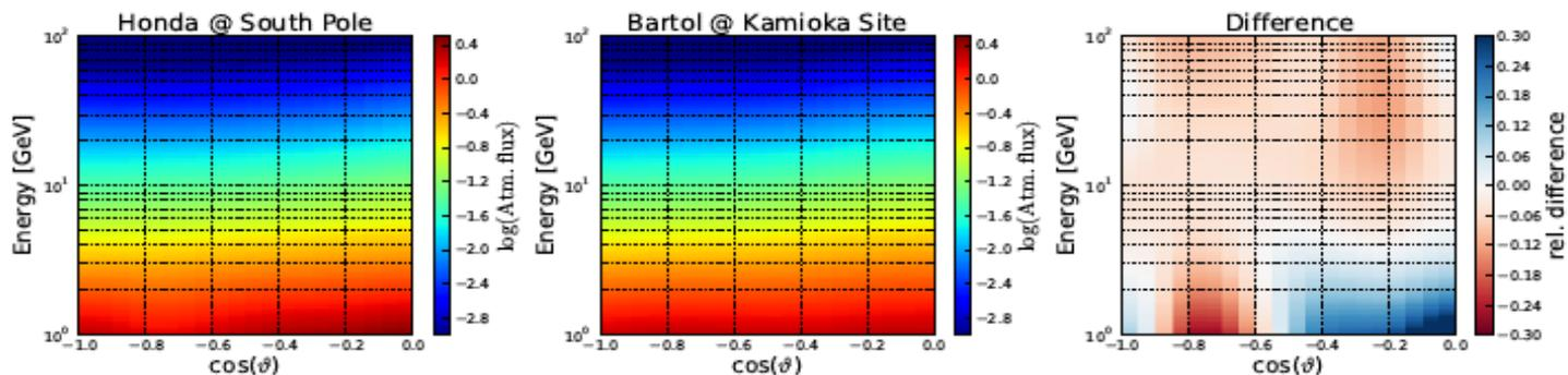
*Comparison of the atmospheric neutrino fluxes used by either analysis. Shown is the **muon neutrino** flux as a function of neutrino energy and zenith angle.*
