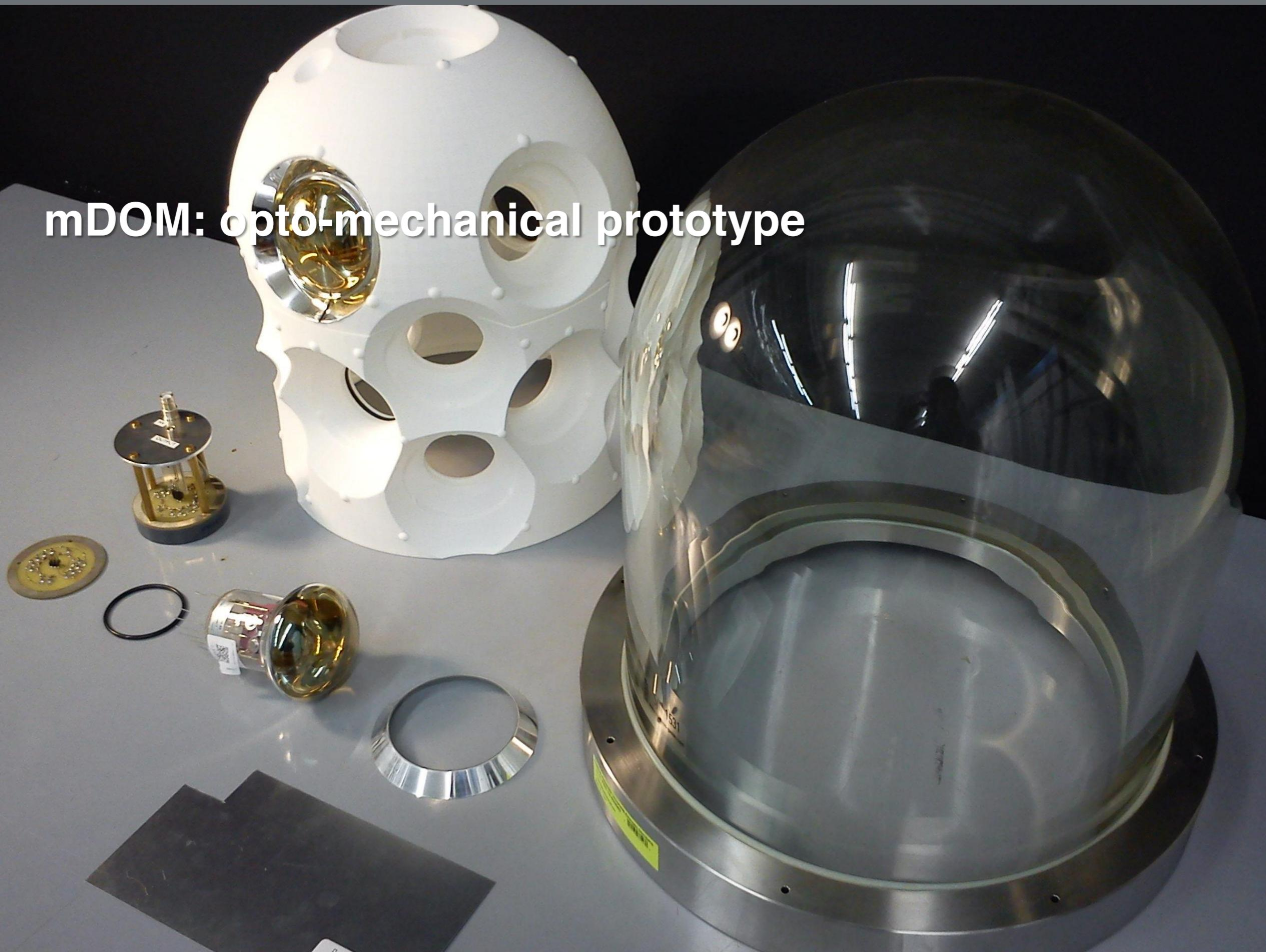
Concept: two 8' PMT back to back in a elliptical glass house
