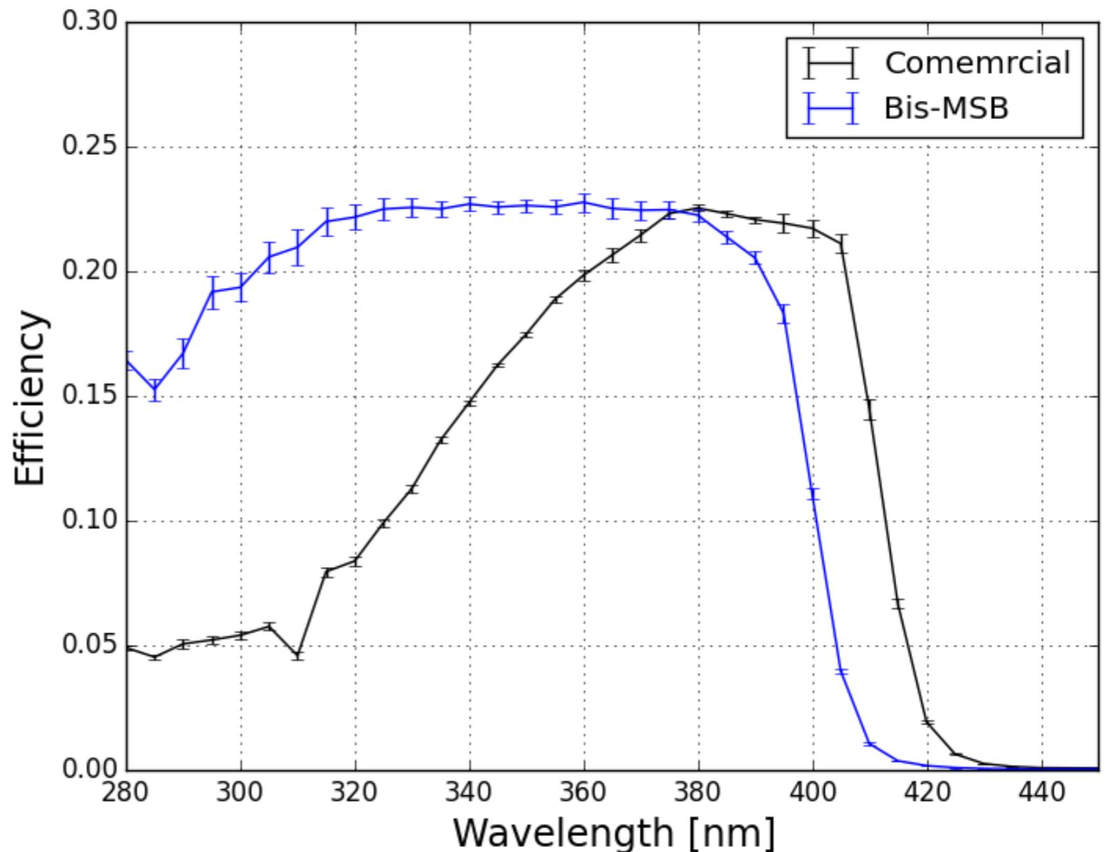
Efficiency includes absorption, re-emission, and light guiding to photosensor
