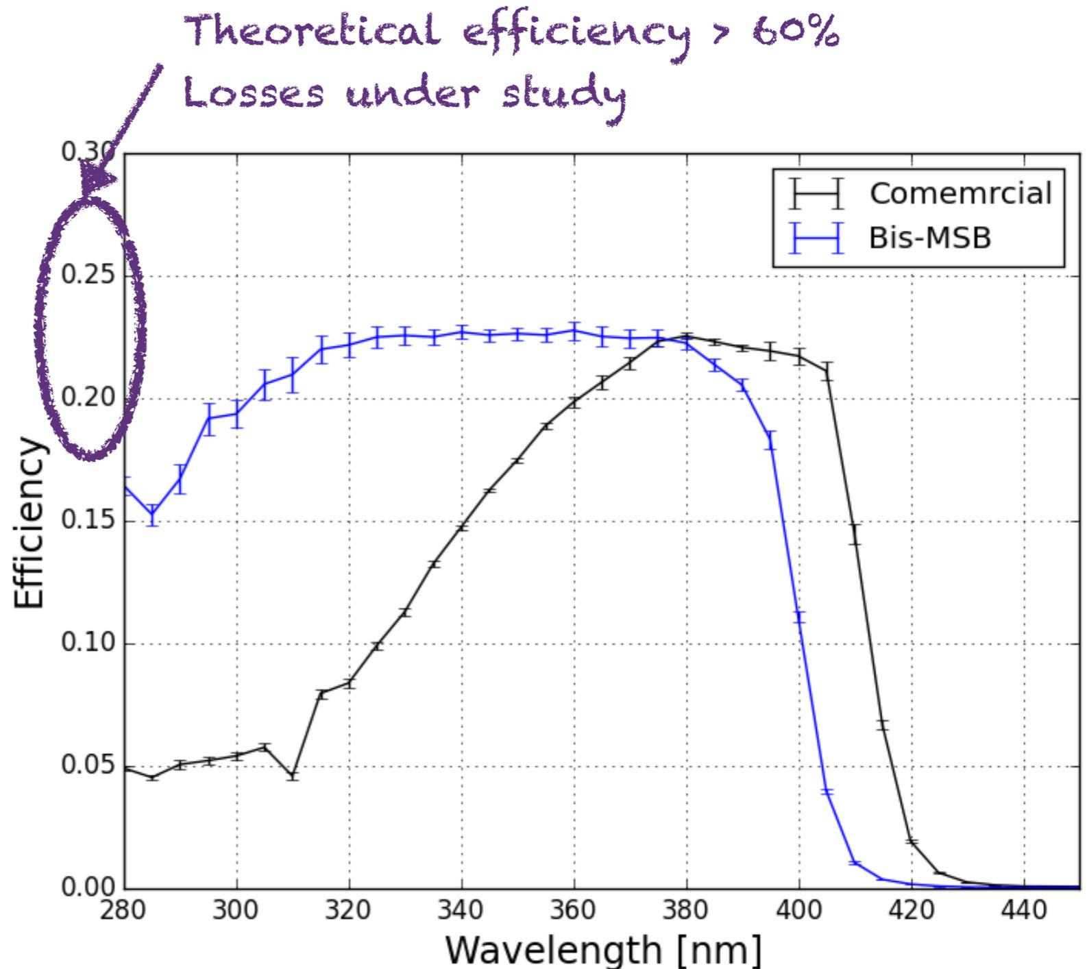
Efficiency includes absorption, re-emission, and light guiding to photosensor
