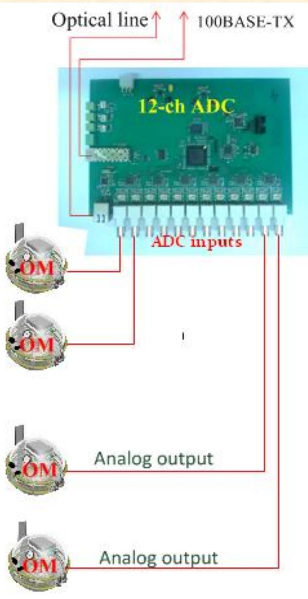
A group of Optical Modules (Section) are connected to one multi-channel ADC board, that provides data processing.
