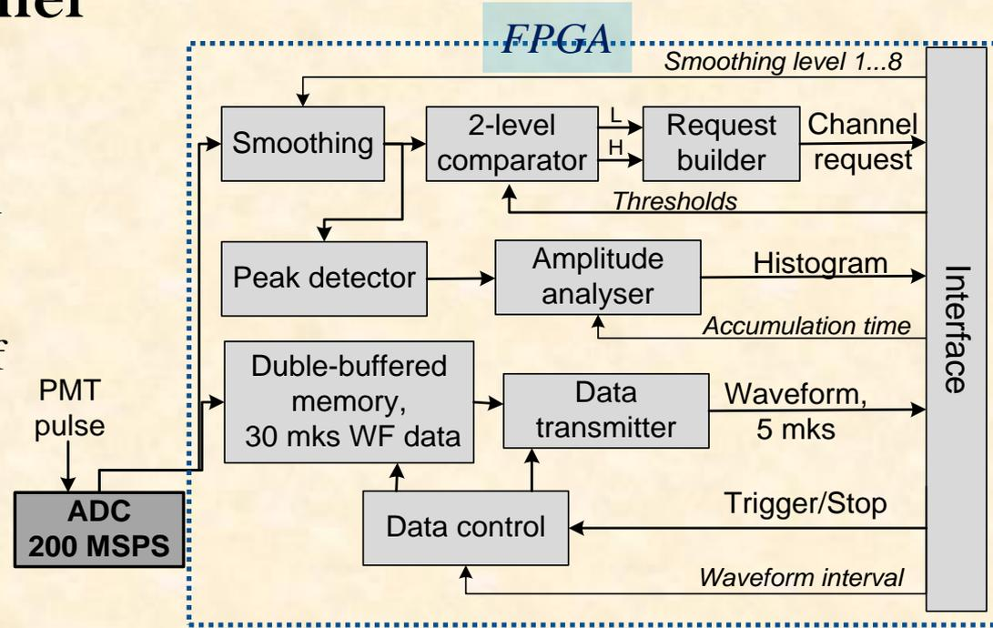
Functional scheme of one FADC channel
