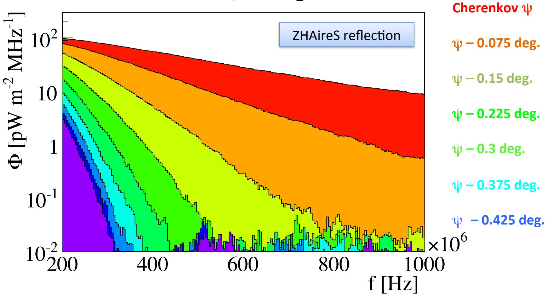
Spectrum flattens as observer moves towards Cherenkov angle
