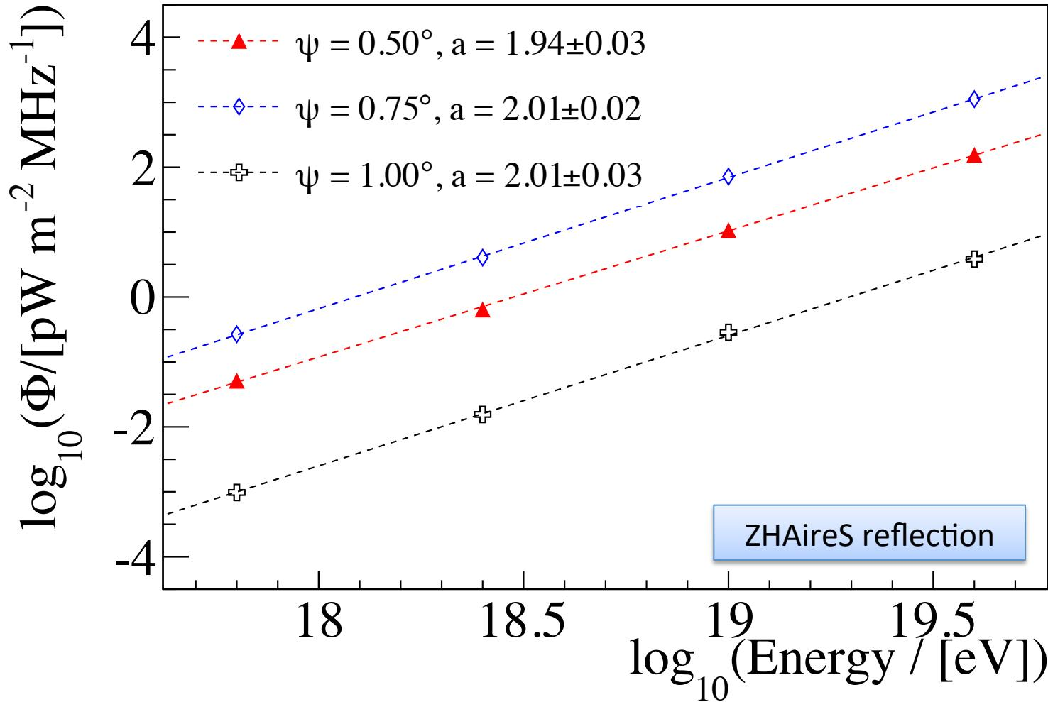
Measuring flux density & off-axis angle (spectral slope) => energy determination
