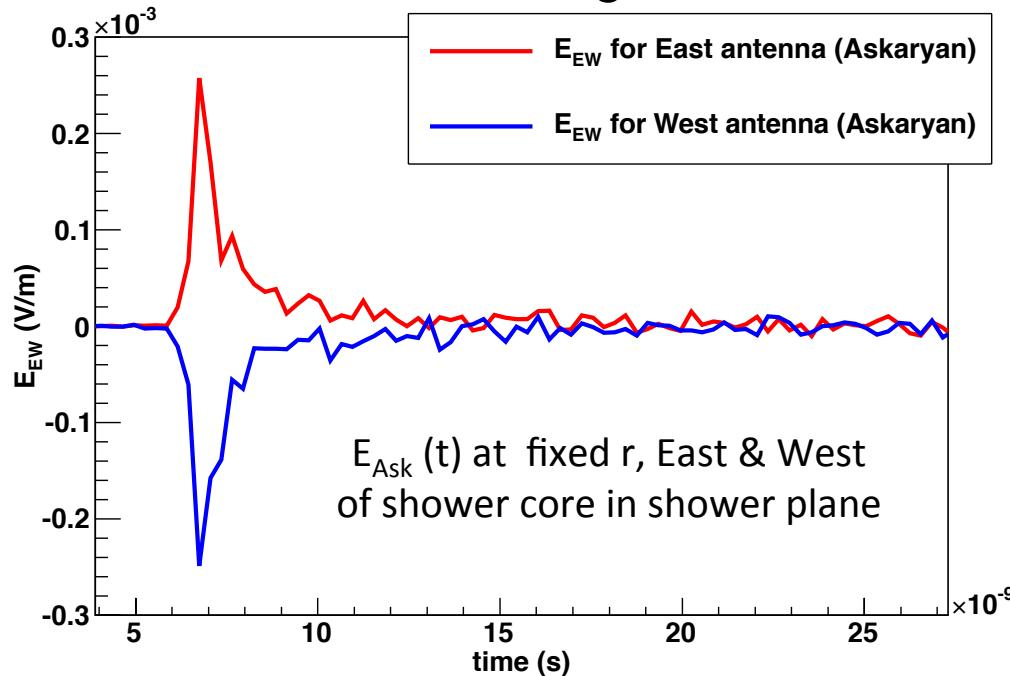
$E_{\text{geo}}(t)$  &  $E_{\text{Ask}}(t)$  circularly symmetric in shower plane even at the level of time traces
