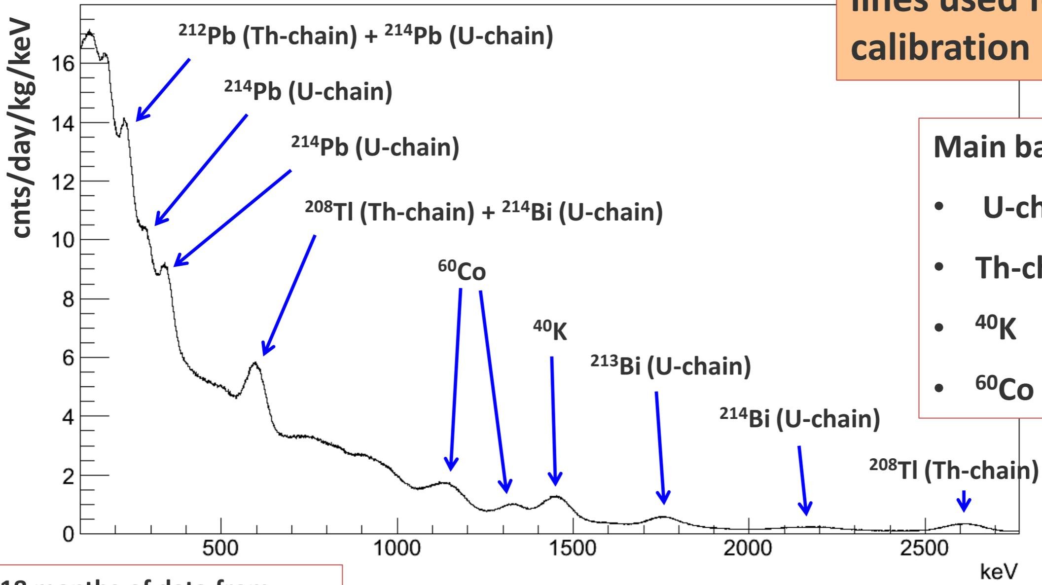
Internal contamination lines used for calibration
