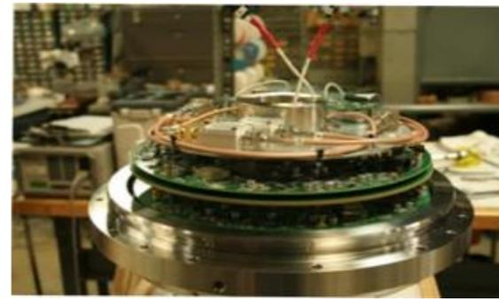
Temp and pressure sensors mounted on the mainboards
