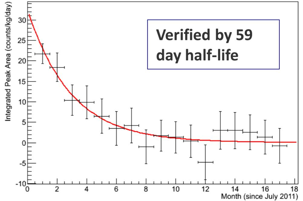
Cosmogenic lines verify our energy calibration; this is particularly useful for the prototype since we do not have an in-ice source.
