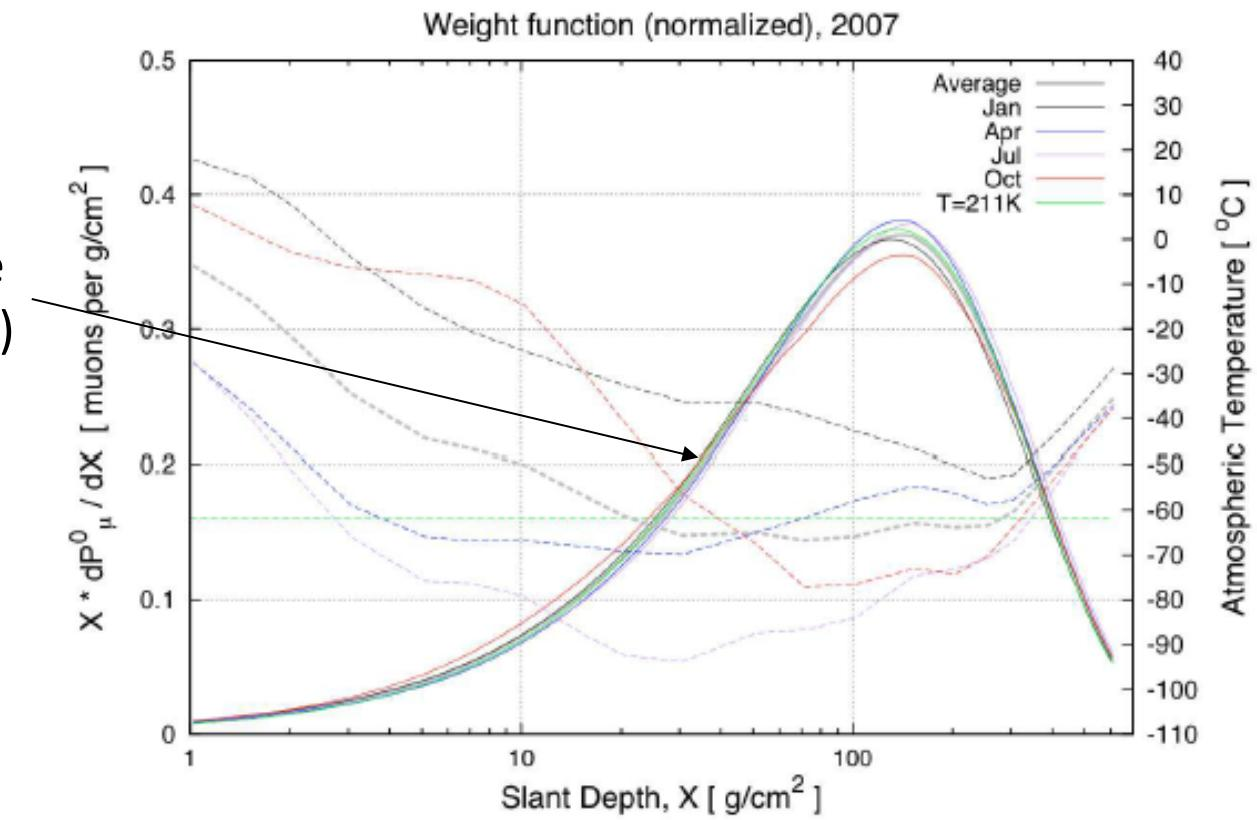
$$T_{\text{eff}}(E_\mu, \theta) = \frac{\int_0^X dX T(X) \mathcal{P}_\mu(E_\mu, \theta, X)}{\int_0^\infty dX \mathcal{P}_\mu(E_\mu, \theta, X)}$$
