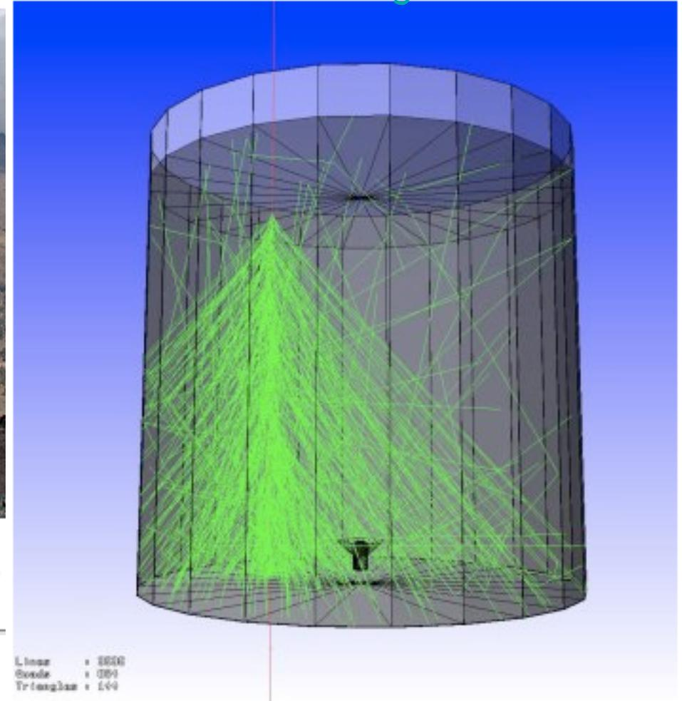
A 5 meter diameter tank as simulated in Geant4 for a single vertical muon. The number of photons are reduced by a factor of 50 for visualization.
