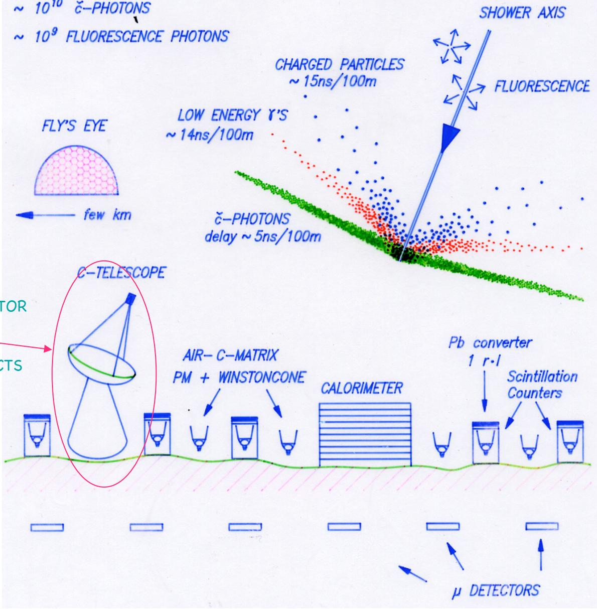
IMAGING CHERENKOV TELESCOPE
