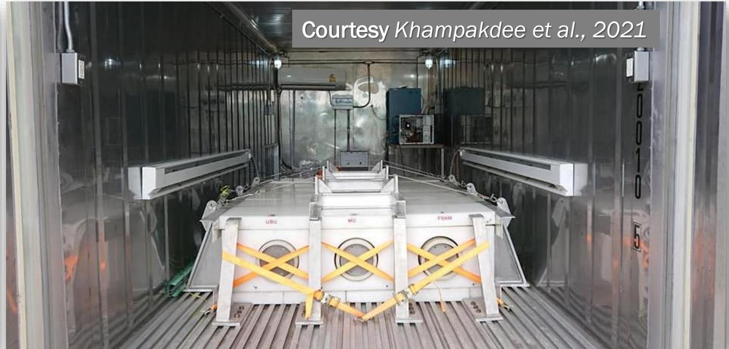
**FIGURE 3** The placement of the semi-led neutron monitor inside the shipping container
